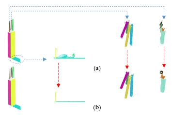
**Figure 6.** Comparison of type II errors during the point-to-model assignment: (**a**) scan vs. BIM with  $\varepsilon_{Const.} = 100$  mm and (**b**) proposed point cloud vs. model.
