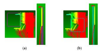
**Figure 8.** Results of heuristic model fitting of a hollow structural section (HSS) to contaminated point clouds using Verity: (a) original registered model and point cloud and (b) result of the incorrect model fitting.
