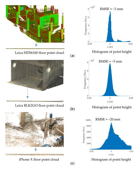
**Figure 2.** Sample point cloud (left) and histogram of point height (right) for (a) Leica HDS6100 terrestrial laser scanner (TLS) [43], (b) Leica BLK2GO mobile scanner [44], and (c) 3D reconstruction using iPhone X images.
