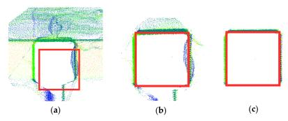
**Figure 15.** Comparison of Algorithms 1–3 with local implementation of scan vs. BIM: (a) sample HSS member (with rounded rectangular edges) and surrounding point cloud with visible local construction error; (b) local scan vs. BIM; and (c) proposed Algorithms 1–3.
