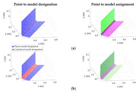
**Figure 14.** Results of the point-to-model designation (left) and final assignment (right) using (a) the random sample and consensus (RANSAC) method of [34] and (b) the proposed method (Algorithms 2 and 3).
