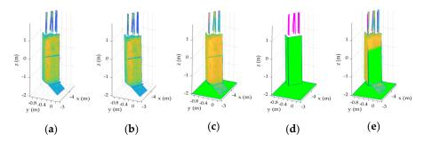
**Figure 4.** Experimental setup for demonstration 1: (a) original point cloud, (b) translated and rotated point cloud, (c) as-built model of the transformed point cloud of Figure 4b superimposed onto the point cloud, (d) as-built model of the transformed point cloud, and (e) as-built model of the transformed point cloud superimposed onto the original point cloud.
