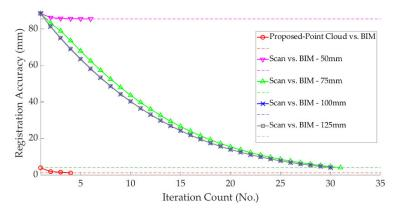
**Figure 5.** Registration error vs. the iteration number using proposed method of Algorithm 1, compared to the result of scan vs. building information modeling (BIM) [20], with  $\varepsilon_{Const.} = 50$  mm, 75 mm, 100 mm and 125 mm.
