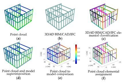
**Figure 1.** Typical framework for automatic assignment of points to the designed multi-dimensional (n-D) information model elements: (a) point cloud, (b) n-D information model, (c) elemental classification of the designed model, (d) superimposition of the point cloud and the model, (e) point-cloud-to-model comparison (in this case, the color represents the distance of the points to the closest element's surface), and (f) result of assignment of the point cloud to the corresponding elements.
