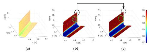
**Figure 11.** Results of the neighborhood definition: (a) sample point cloud, (b) Weinmann's [26] method, and (c) using Algorithm 3.
