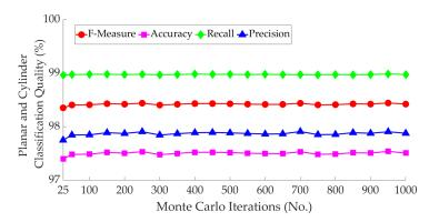
Figure 12. Quality of point-to-model designation using Algorithm 2 vs. the number of iterations.
