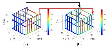
**Figure 7.** Distance of the point to the 3D element model using (**a**) only the initial reliable target-based registration and (**b**) the iterative closest point (ICP) fine registration [20].
