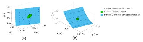
**Figure 3.** Schematic intersection of a sample ellipsoid with a 3D model: (a) planar surface and (b) cylindrical surface.
