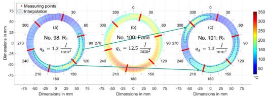
Fig. 7 High-resolution temperature measurement with fiber optics (a) before; (b) during; and (c) after fade.
