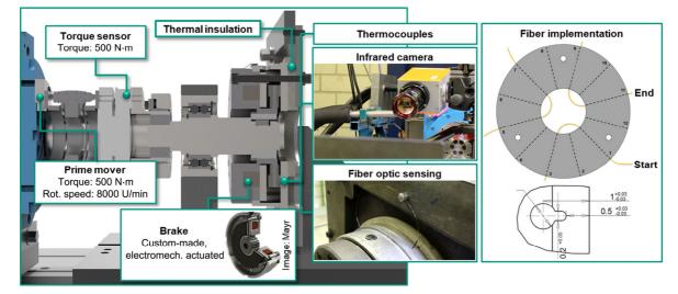
Fig. 2 Test setup brake with fiber optics and infrared technology.
