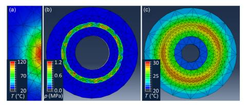
**Fig. 10** Results of the 3D FEM simulation. (a) Temperature in the cross-section of the ideally smooth disk with rotationally symmetrical temperature distribution; (b) surface pressure with asperities; and (c) temperature of the surface with asperities after 14 s of cooling [38].
