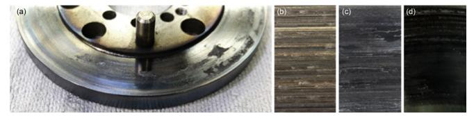
Fig. 17 More examples of material transfer. Pictures of (a, b) steel disks of mass pressed; (c) wound; and (d) sintered metal friction linings.
