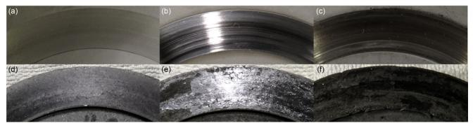
Fig. 11 Steel disk (top) and friction lining (bottom); after running-in (a, d); after fade (b, e); and after recovery (c, f).
