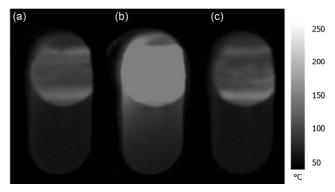
**Fig. 9** Thermography measurement of the friction lining (a) before; (b) during; and (c) after fade.
