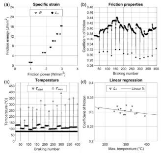
**Fig. 4** Determination of the fade limit. (a) Specific strain of the reference and load levels with gradual increase; (b) coefficient of friction of each brake cycle with drops during the load levels; (c) start and maximum temperatures of each brake cycle with increase during the load levels; and (d) correlation between the maximum temperatures and the coefficient of friction.
