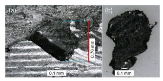
**Fig. 16** Detached plateau with (a) a smooth and shiny upper side and (b) a rough and dull bottom side.
