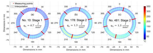
Fig. 6 High-resolution temperature measurement with fiber optics in (a) early; (b) mid; and (c) late brake cycles of the running-in.
