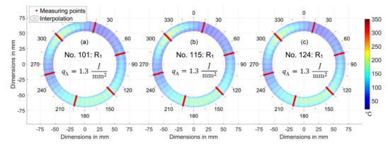
Fig. 8 High-resolution temperature measurement with fiber optics (a) five; (b) fifteen; and (c) twenty-four cycles after fade.
