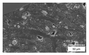
**Fig. 1** Cross-section of the friction lining in the scanning electron microscope.
