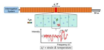
**Fig. 3** Using Rayleigh scattering and converting its frequency shift in order to evaluate temperature or strain, redrawn from [31].
