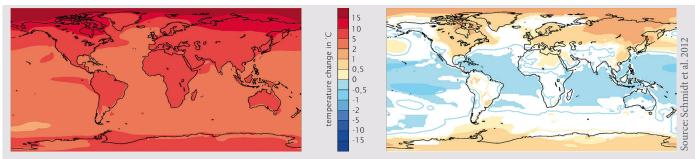
Modelling of temperature changes in the climate scenario with a  $CO_2$  concentration four times higher than the pre-industrial level (left) and in the scenario of the application of RM technologies to maintain the pre-industrial global average temperature despite the high  $CO_2$  concentration (right). A uniform temperature reduction through RM measures would probably not be achievable; the consequence would be overcooling of the tropics and warming of the polar regions.
