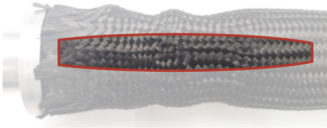
Fig. 7: Formation of Wrinkles in first draping experiments.
