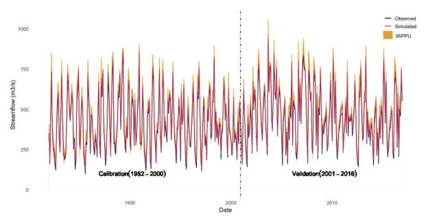
Figure 3-8: Uncertainty analysis with SUFI-2 algorithm for calibration and validation of streamflow
