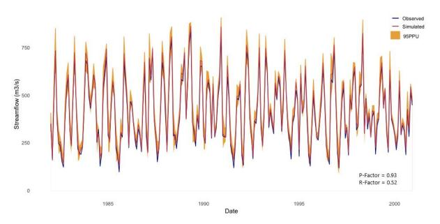
Figure 3-9: Calibration of the model and Uncertainty analysis of monthly streamflow (m<sup>3</sup>/s)
