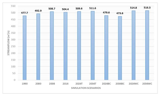
Figure 3-12: Average daily streamflow (m<sup>3</sup>/s) that reaches the HPP at the catchment outlet by scenario.
