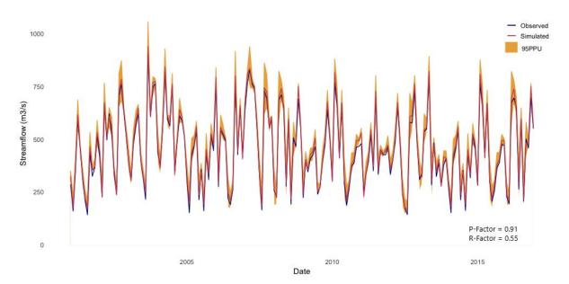
Figure 3-10: Validation of the model and Uncertainty analysis of monthly streamflow (m³/s).
