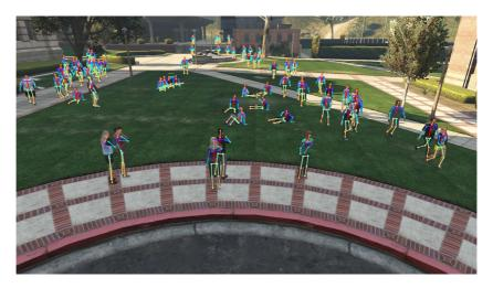
**Figure 3.2**: Synthetic crowded scene. SyMPose consists of around two dozen scenes showing different places filled with many people. All scenes are recorded from a higher-level camera that should simulate the target scenario in urban settings. The underlying skeleton model consists of a subset of the JTA model and was designed to mimic the model used in CrowdPose [5].
