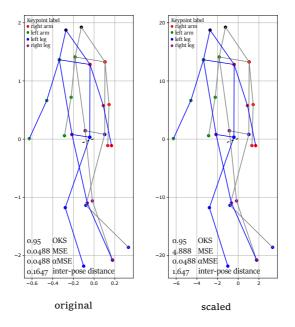
**Figure 4.1**: Visual and quantitative comparison for poses at different scales and the effects on the evaluation metrics OKS and MSE. Inter-pose distance and MSE are directly effected by the rescaling of poses, whereas OKS and  $\alpha$ MSE stay the same due to their scale invariance.
