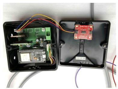
Figure 5.8: Developed board for the learning controller implementation.
