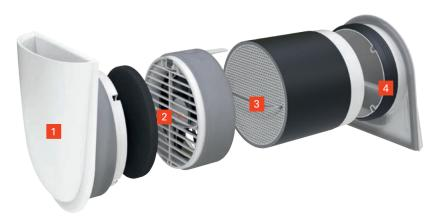
Figure 1.3: Exploded axonometric of a DVS [216]. 1 - Indoor panel. 2 - Reversible fan. 3 - Heat storage system. 4 - Outdoor panel.
