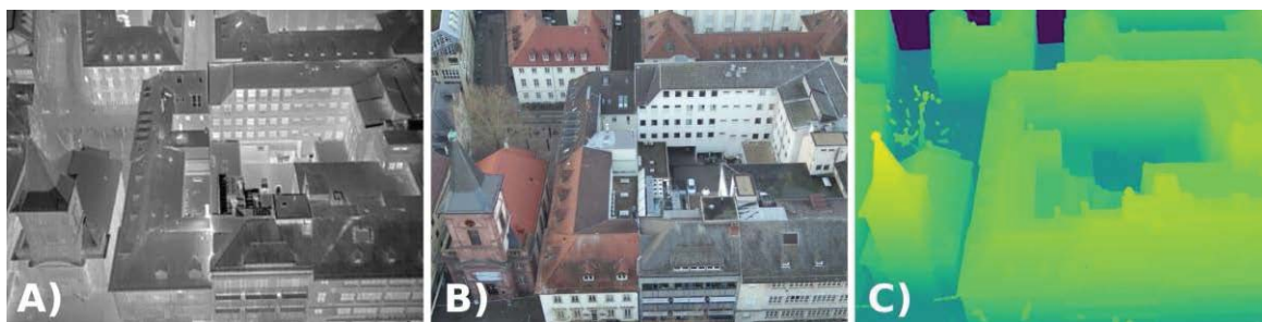
Figure 1: Drone images of the city centre of Karlsruhe used for the TBBR dataset A) thermal image B) RGB image C) image with height information (height map)
