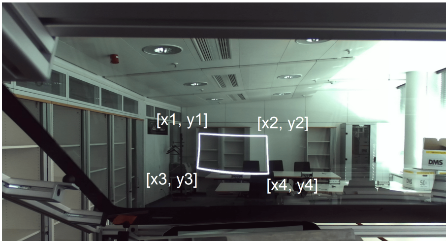
Figure 4.14: Target-free estimation of HUD’s focal lengths. The virtual image frame is rendered and captured by the smartphone camera. All the [x_k, y_k]^T ( k \in \{1, 2, 3, 4\} ) represent its corner positions. Note that the expected rectangular virtual image enclosed by the white margins is distorted.
