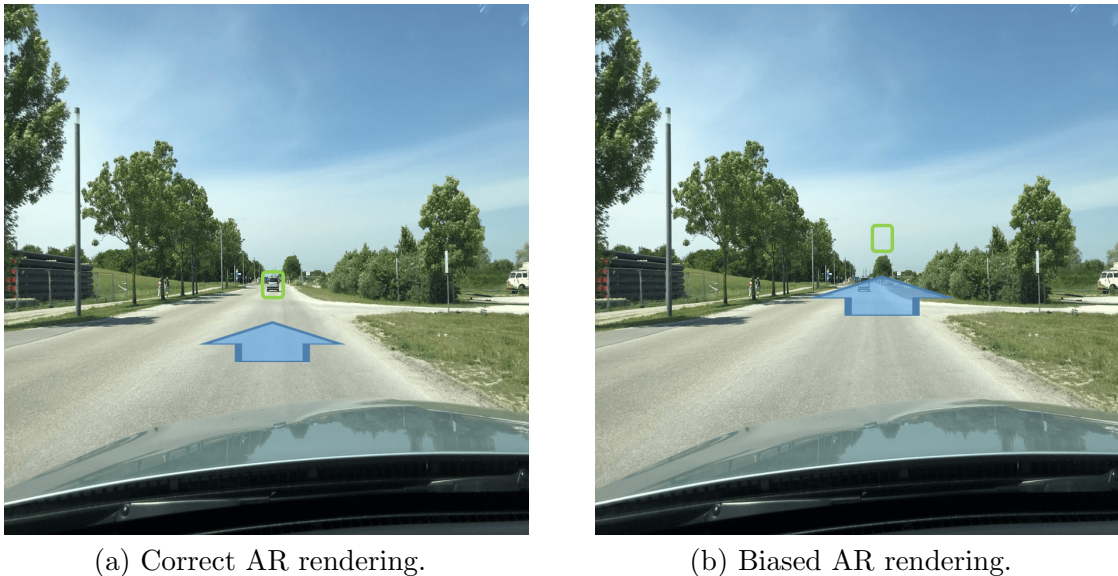
Figure 1.2: Illustration of virtual objects (e.g. a blue navigation arrow and a green vehicle tracking box) presented by a precisely calibrated AR-HUD (a) and a biased one (b). Compared to the correct AR rendering via a calibrated HUD, that from an uncalibrated or wrongly calibrated HUD may lead to deviated navigation or occlusion.
