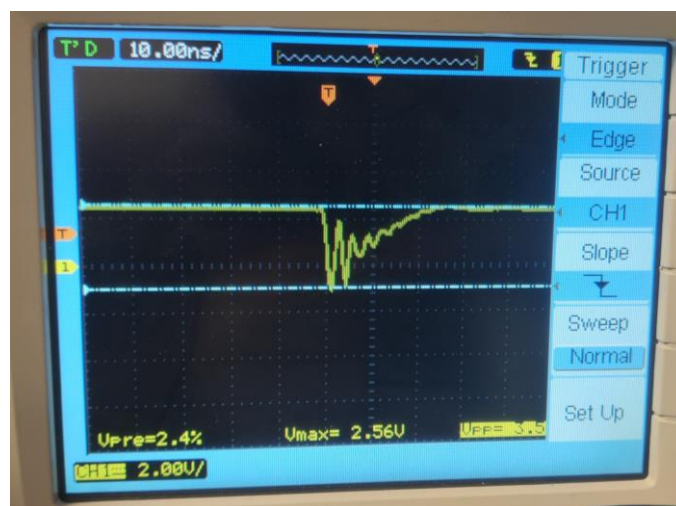
Fig. 17. Initial pulses generated showing heavy ringing
