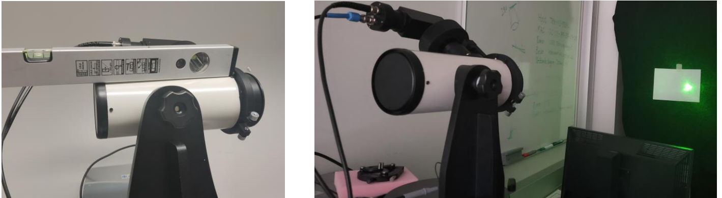
Fig. 31. Experimental setup to confirm the sensor FOV for the MSL
