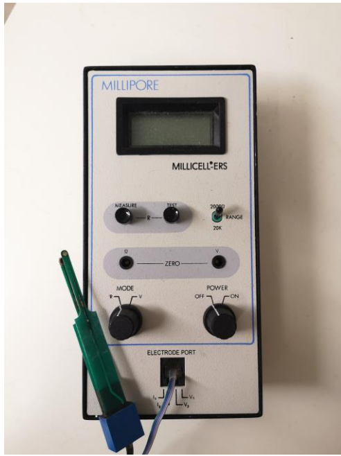
Figure 8: The Millicell®-ERS with connected electrodes used for measurements of the transepithelial electrical resistance (TEER).
