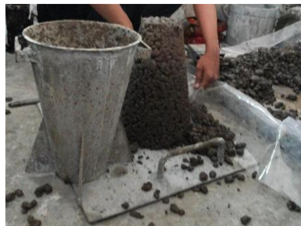
(b) Poor workability
