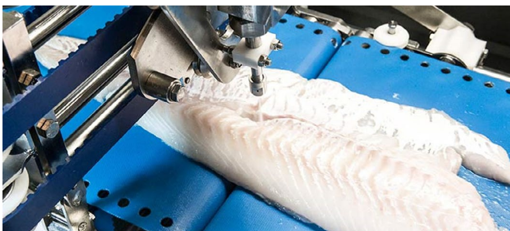
Figure 14. Marel flexicut machine uses high-pressure water to cut fillets into portions or remove bone and belly flaps
