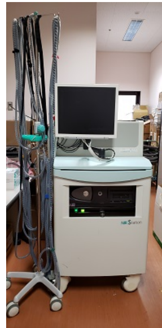
Fig. 1. The image of the OMM-3000 device used to record brain activities.
