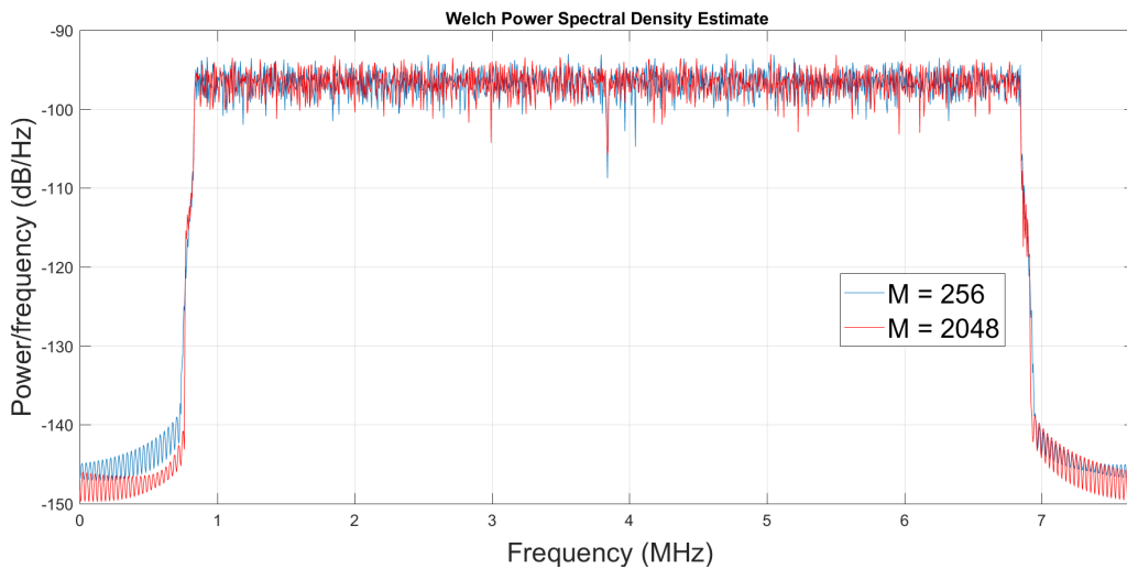
Figure 5.6: Comparison between two fOFDM signals in the frequency domain with different filter orders. Notice how the spectrum decay is faster for the higher order filter.
