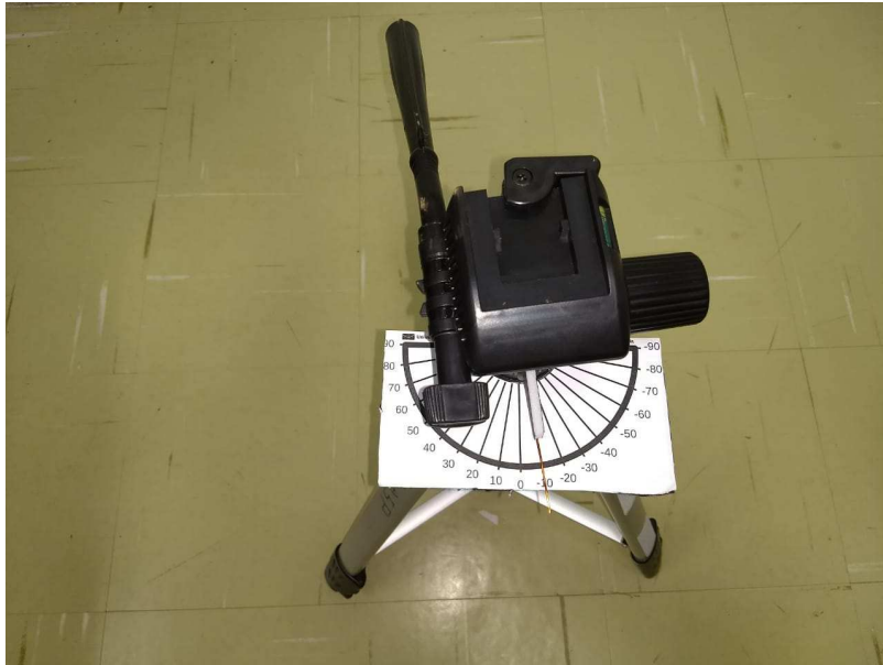
Figure 3.5: Protractor used to verify the rotation of the receiver base. There is a precision error that becomes larger for larger values of |\theta| .
