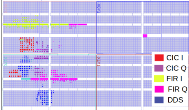
Figure 8. Layout of the routed circuit highlighting the resource occupancy of each submodule.
