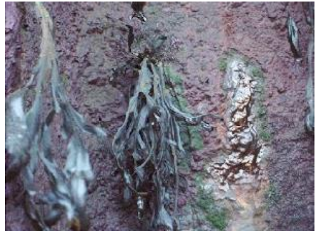
Figure 2-8 MIC formation without tubercle (Beech and Campbell, 2008)
