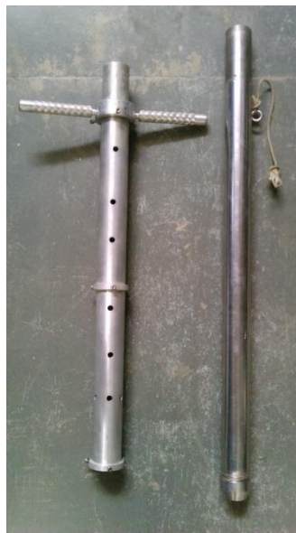
Figure 3-5 Corer head with extension tube
