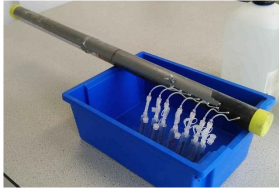
Figure 3-6 Sediment corer sleeve with Rhizon samplers fitted
