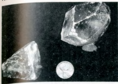
Shows variation in crystal habit (note the tendency for rhombohedral cleavage on broken surfaces).
