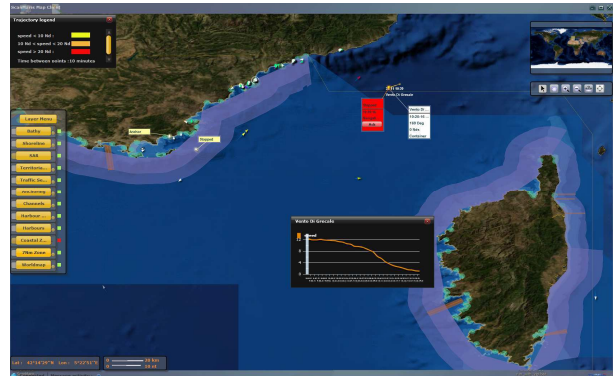
Figure 5. Alarm on container propulsion failure with vessel location and date (red vignette), vessel type and name (white vignette) and speed history profile (black vignette)
