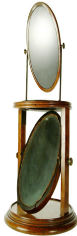
Fig. 9. Polariscope. Christian Norremberg, 1830, University of Glasgow, http://collections.gla.ac.uk/#/details/ecatalogue/3898
