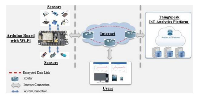
Figure 2. The architecture of an IoT-based monitoring and control system
