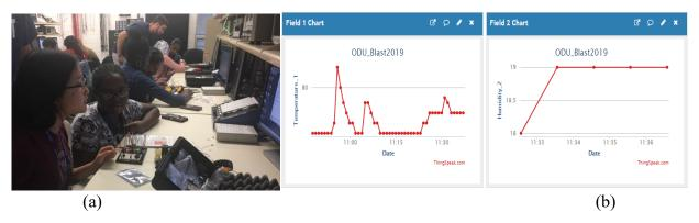
Figure 3. (a) Student working on IoT hands-on activities and (b) a screenshot of ThingSpeak user interface showing temperature and humidity sensor data
