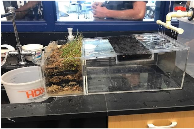
(a) Unit with a mixed-media bio retention system.
