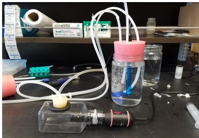
Figure 6. Experimental setup for the acidification session, including a pH probe inserted through a stopper into a glass jar into which \text{CO}_2 was allowed to flow, and a \text{CO}_2 sensor that measured \text{CO}_2 concentration in the air that was displaced from the glass jar.
