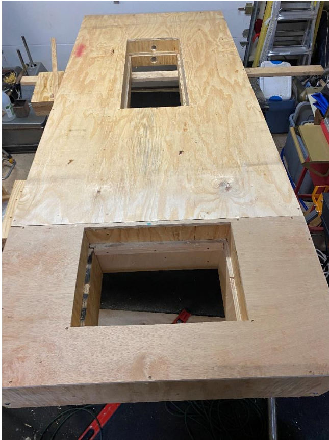
Figure 4. Mound surface structure. The mound surface structure was built with overlaid sheets of 3/4-inch thick plywood and cut using a circular saw.
