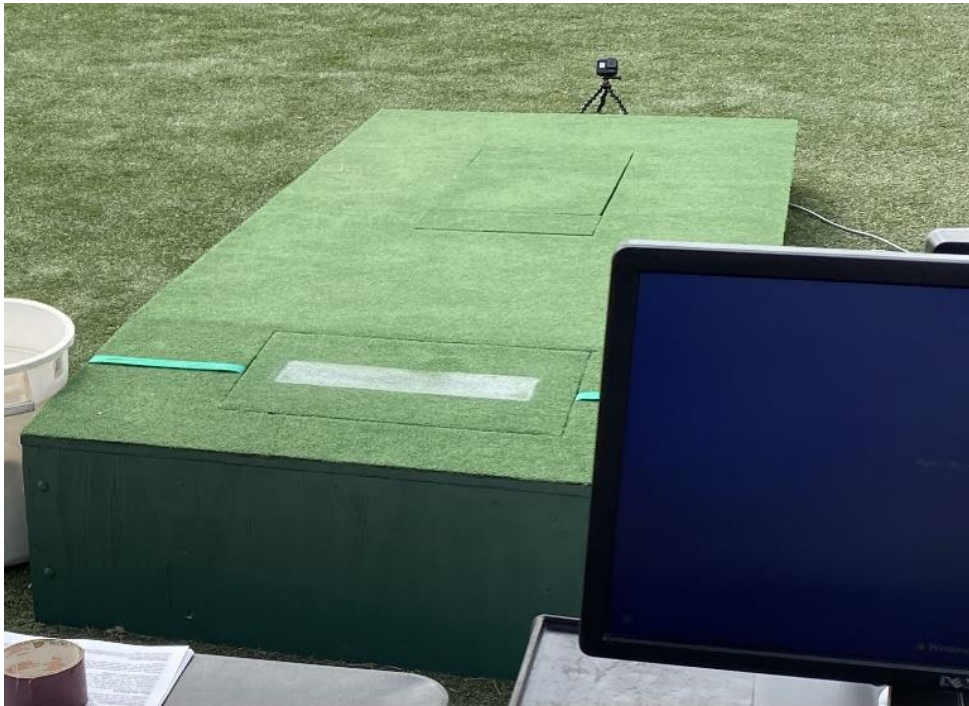
Figure 7. Outdoor laboratory setup. The instrumented pitching mound was setup outside during each day of data collection.
