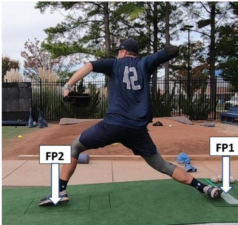
Figure 8. Mound framework. The force plate on the flat shelf of the mound where the pitcher's drive leg is located was labeled as FP1, and the force plate on the sloping section where the stride leg lands was labeled as FP2.
