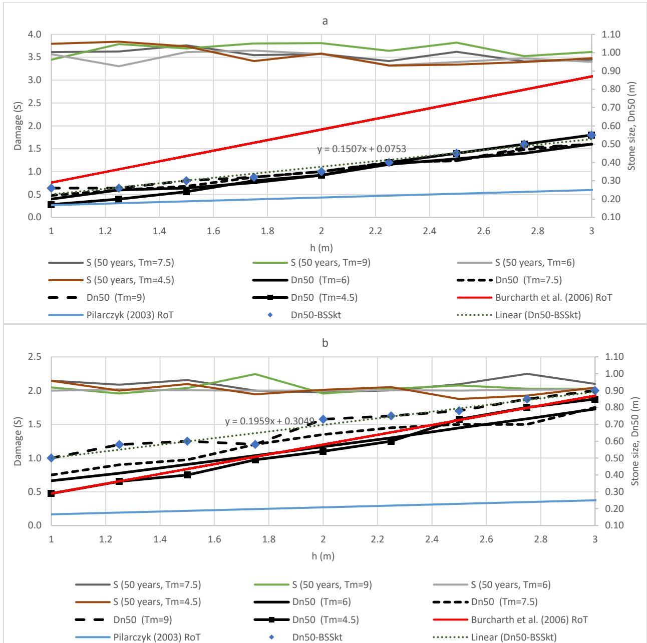
Figure 5.19. Predicted stability of LCS for S < 2 at N_w = 3,000 , and S < 4 for N_w to 15,500 (a) and S < 2 at N_w = 15,500 (b).
