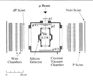
FIG. 1. The experimental arrangement. Shown are the two identical charged-particle detection systems on either side of the  ${}^{3}$ He gas cell in which the muons are stopped.
