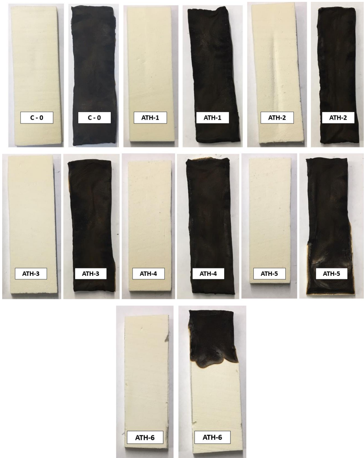
Figure 3.44. Digital images for the flame retardant rigid polyurethane foams containing ATH before and after the burning test.
