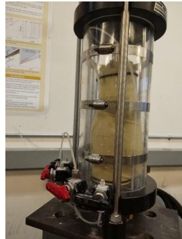
(b) Shear failure
