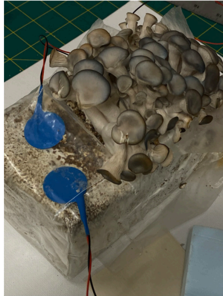
Piezo disc, Contact mic on blue oyster mycelium (LM386 Amplifier connected)
