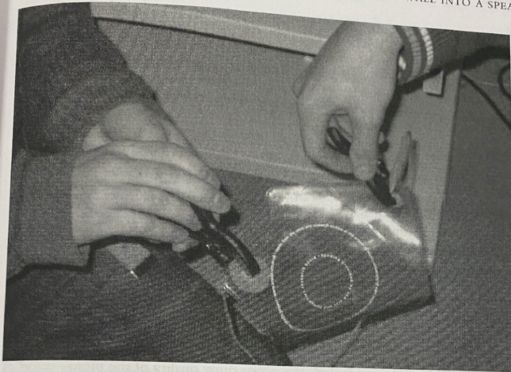
Figure 8.3 A piezo driver and contact mike pickup being used to filter a sound through a sheet of plastic.
