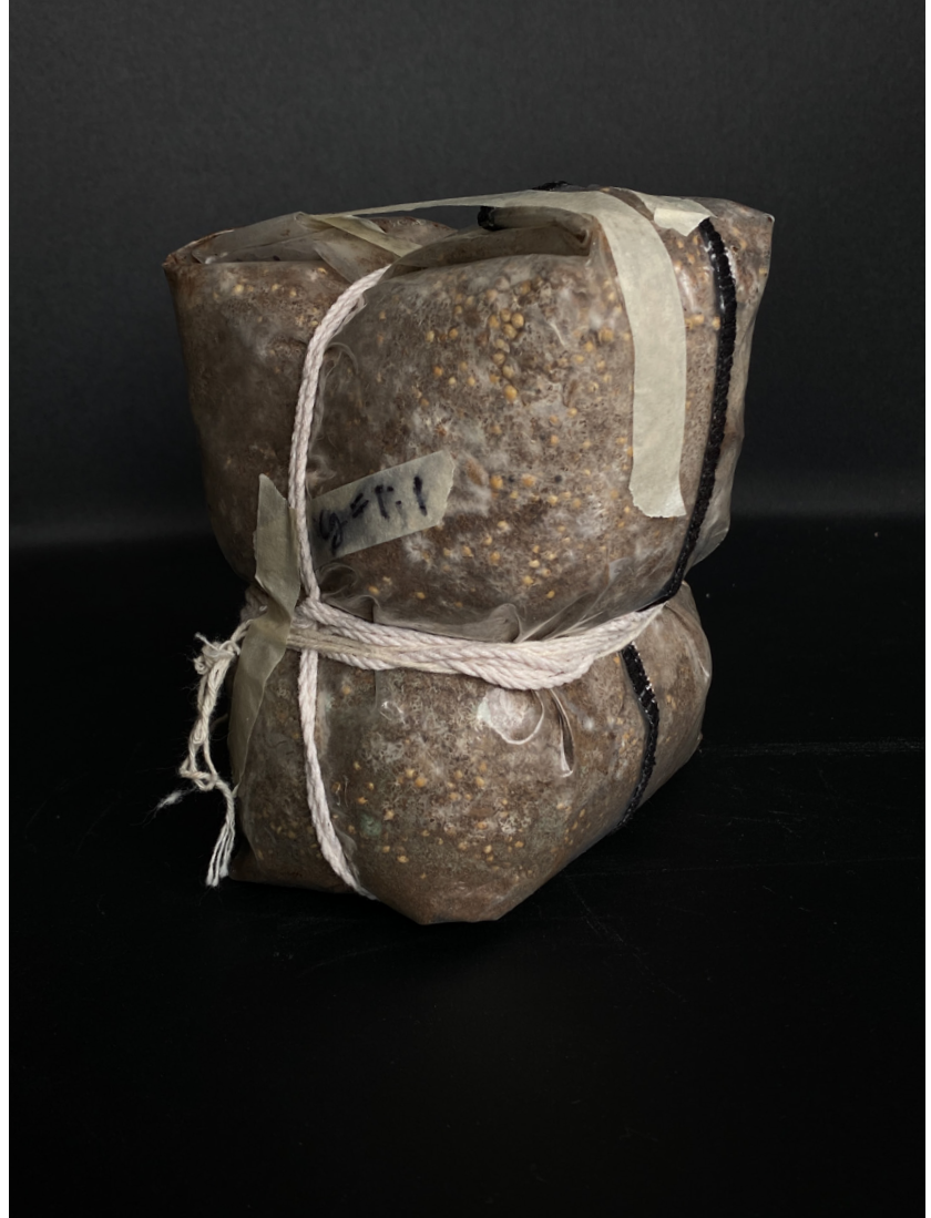
First mold test - Growing mycelium with used coffee grounds and white millet (3/17/21)
