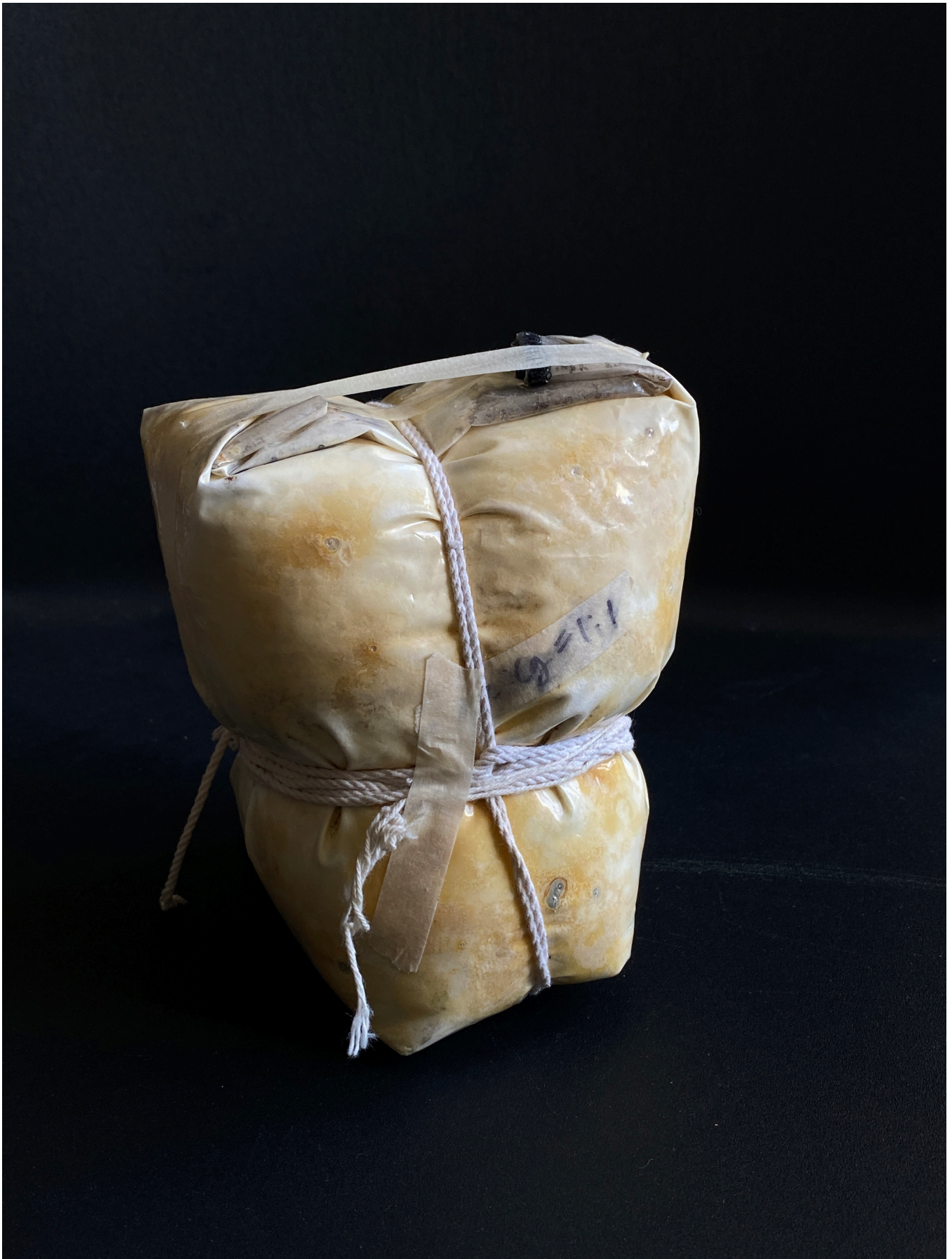
First mold test - Growing mycelium with used coffee grounds and white millet (4/17/21)
