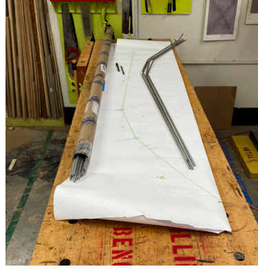
Each of the aluminum rods was bent using a clamp and measured against the pattern.
