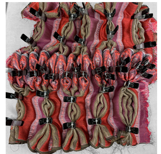
After steaming the textile is folded and secured using clips for 24 hours.
