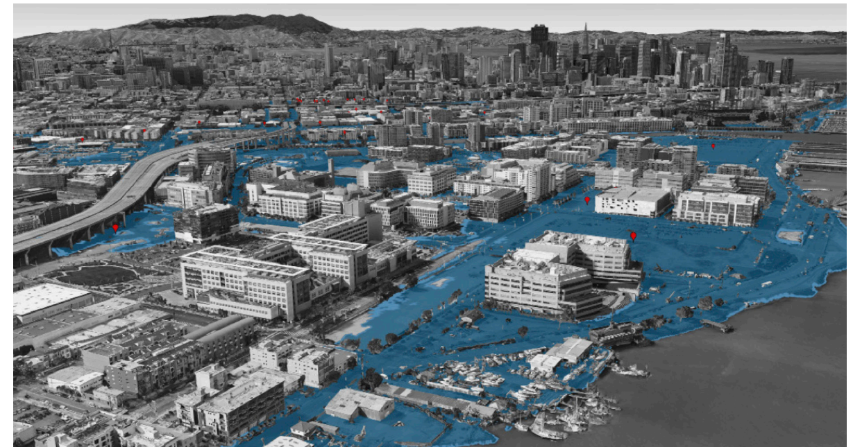
Much of Mission Bay and South of Market could flood by 2100 if sea rise and storm surge exceed 8 feet above current high tide, as some models predict. Red points indicate new development projects, including the Golden State Warriors Arena and Mission Rock mixed-use development. Illustration by Marcea Ennamorato & HyunJu Chappell, 2017, Public Press, San Francisco, CA.
