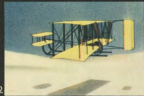
2 . . . Kittyhawk, California. The plane had 4 cylinders, a 12 h.p. motor and chain-driven propellers but—it flew.
