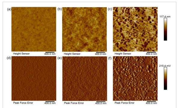
**Figure 2.** AFM images of phase and topography for (a) and (d) pristine PffBT4T-C9C13, (b) and (e) unannealed PffBT4T-C9C13:PC $_{70}$ BM (1:1.2) and (c) and (f) annealed PffBT4T-C9C13:PC $_{70}$ BM (1:1.2) blend film. Scale bars are 400 nm.
