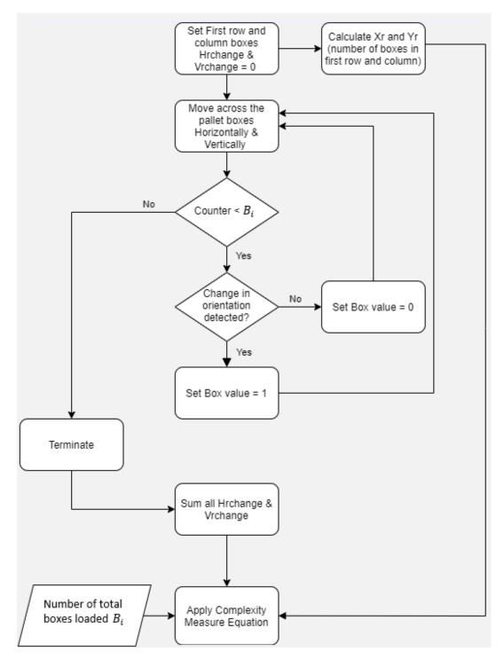
Figure 2.4: Complexity Measure Flowchart
