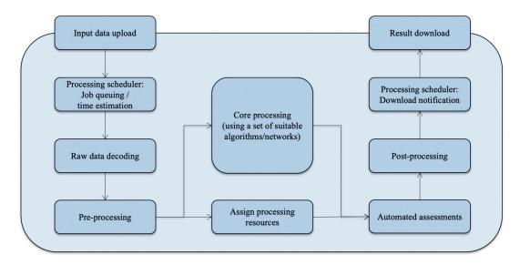
Figure 18. Proposed future streamlined SRR processing system based on automated SRR and quality assessments.
