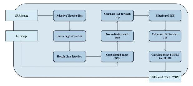
Figure 4. Flow diagram of the proposed ELF automated image effective resolution assessment system.
