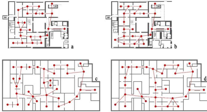
Figure 5: Unjustified graphs of the MoMA. (a) 2005 Fourth floor; (b) 2005 Fifth floor; (c) 2019 Fourth floor; (d) 2019 Fifth floor
