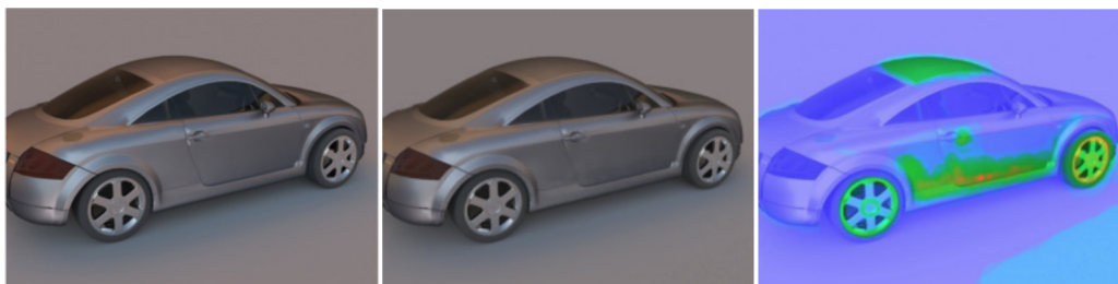
Figure 2.5: Visibility map (on the right) shows the probability of detecting the differences between a reference image (on the left) and a distorted image (in the middle).
