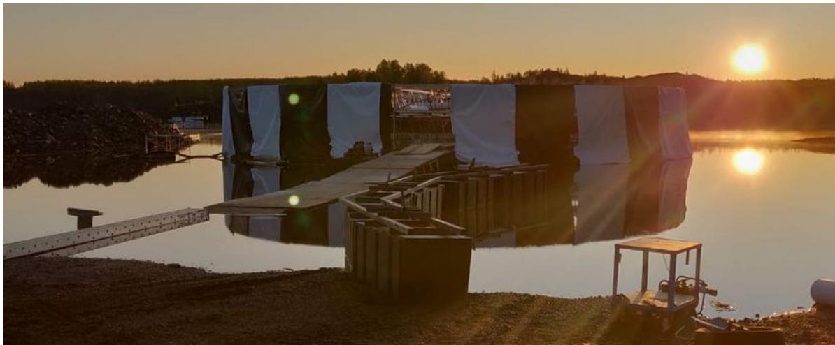
Figure 3.19: Picture of the CHIPS-5 detector module with liner welded up to the height of the top-cap. A section of the floating-dock can also be seen in the foreground.
