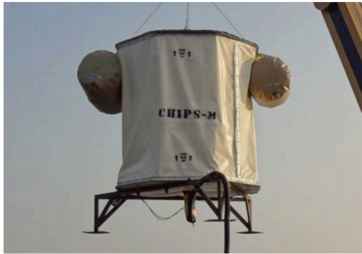
Figure 3.1: Picture of the 3.3 m high CHIPS-M detector just before deployment. Temporary floatation bags are attached to the top rim of the detector, while the umbilical cord carrying data, power, and filtered water is attached to the base.
