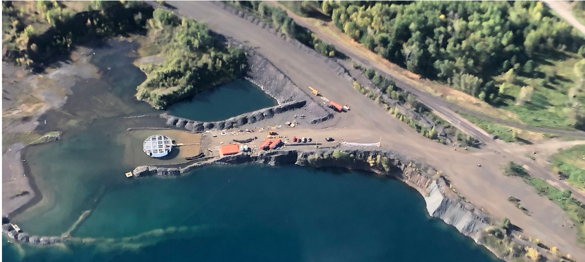
Figure 3.10: Aerial picture of the CHIPS-5 construction site facing south. The Wentworth 2W pit is in the lower half of the image, with the part built CHIPS-5 detector visible at the bottom of the earthen construction ramp. The two white shore huts can be seen halfway up the ramp.
