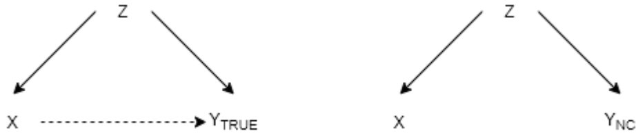
Figure 5.2: Outcome negative control design expressed as a causal directed acyclic graph (DAG). The DAG on the left shows the main analysis. The dashed line between the exposure X and the outcome Y_{TRUE} is the hypothesised causal relationship, which is assumed to be confounded by factors Z . The analyst attempts to adjust for Z in the statistical analysis, but this may or may not be successful. The DAG on the right shows the negative control analysis. By assumption, there is no causal relationship between the exposure and the negative control outcome, Y_{NC} , but there is confounding through Z . If there exists an association between X and Y_{NC} after attempting to adjust for Z (as in the main analysis), the association is assumed to be spurious, providing evidence that the main analysis is confounded.
