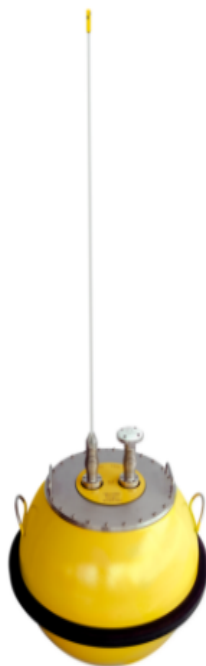
Figure 3.5: An image of the Waverider buoy – the observed long antenna is used for transmitting and receiving GPS signal.
