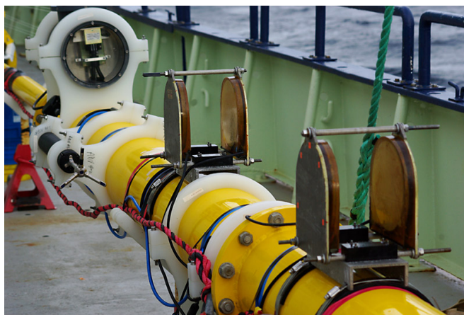
Figure 3.10: An image with the two resonators strapped to the spar buoy before deployment, showing the pairs of transducers.
