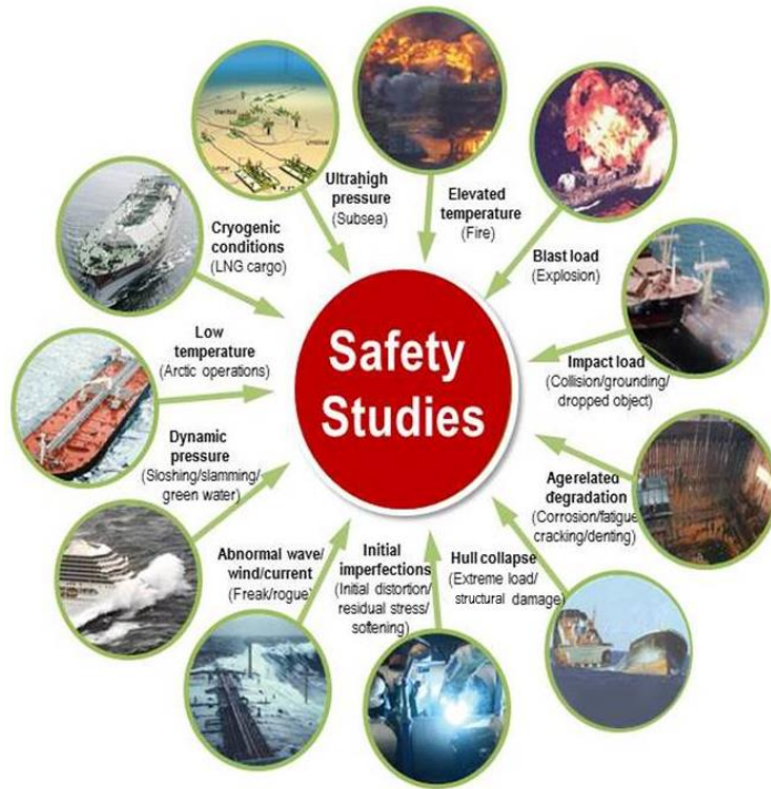
Figure 1.1. Extreme and accidental events involved in ships and offshore structures.
