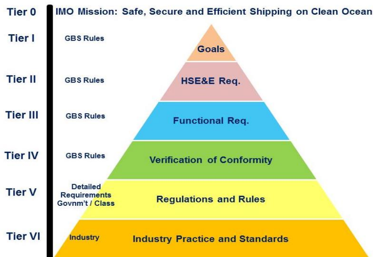
Figure 1.3. Modifications to the IMO’s original concept of GBS with six tiers suggested by Paik (2015).
