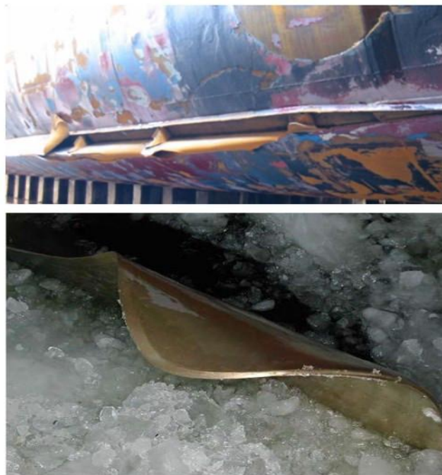
Figure 1.1 Sea ice damage for ship's hull and propeller
