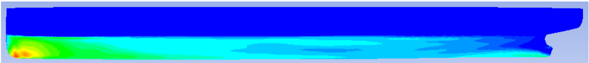
Fig. 5-17 Distribution of dynamic pressure on hull surface at head tilt of 0.1623^\circ
