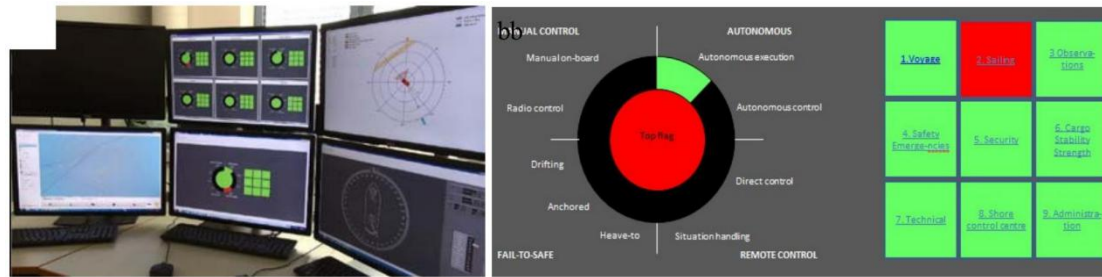
Figure 3-The operator' s workstation and one dashboard to display 9 group information from one unmanned ship
