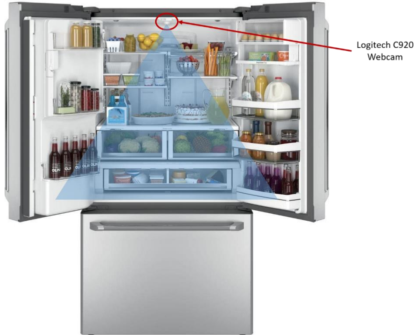
Figure 12. Camera location in the refrigerator and corresponding field of view.
