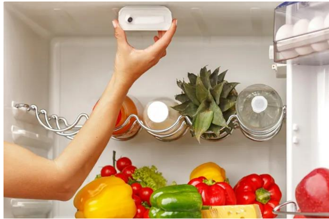
Figure 11. FridgeEye, the battery-operated camera and automatic detection system to make any refrigerator a smart refrigerator.
