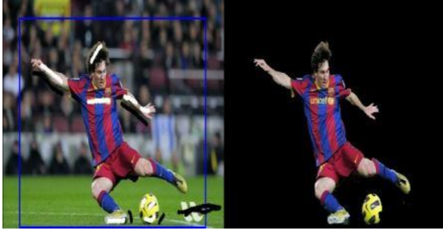
Figure 26. Left: The input image and blue rectangle provided to the program to designate the foreground. Right: The output of the algorithm. [111]
