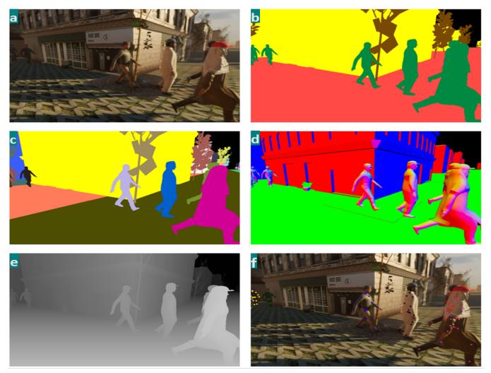
Figure 9: *Silver* provides RGB frames (a) with pixel-level accurate ground-truths for semantic segmentation (b), instance segmentation (c), normal maps (d), depth maps (e), and human body pose information (f).
