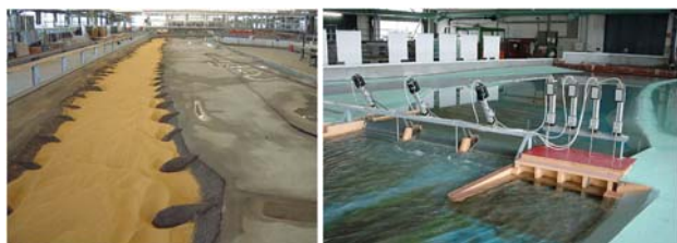
Figure 1. Test bed of a river model, pointwise gauge measurement (source BAW)
