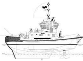
Figure 10: Tug Outboard Profile
