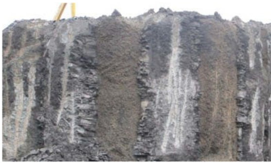
Figure 2: Result of a large-scale test above groundwater level with primary piles made of porous concrete and secondary piles made of usual saturated concrete.
