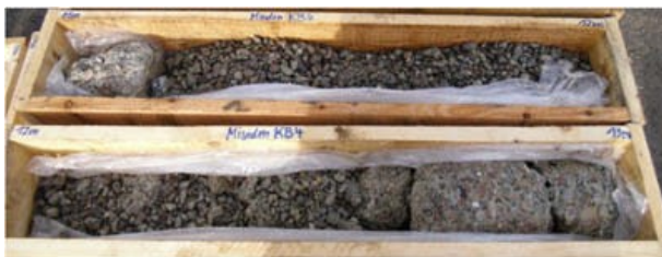
Figure 3: Core result with separated gravel at the top and tight cement stone at the bottom
