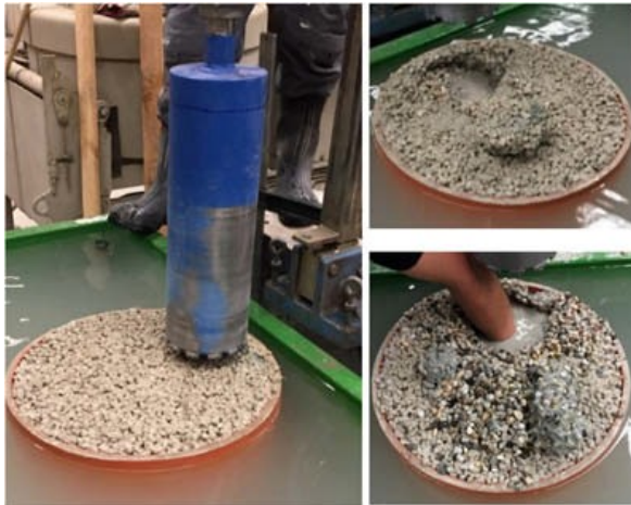
Figure 6: Core-sampling trial after 2 days curing time under water – not successful!
