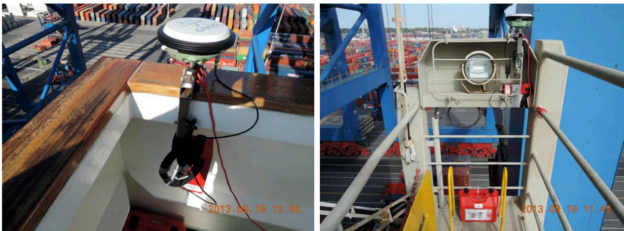
Figure 4.6: GNSS antennae on bridge (l.) and at stern (r.)
