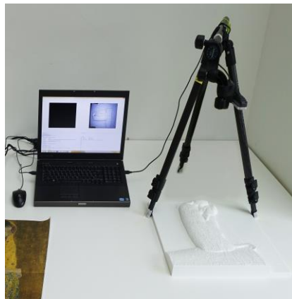
Figure 1: Original hardware setup for testing the context sensitive tactile audio guide for works of art – tactile relief on the right hand side, depth camera positioned above, laptop with debug screen on the left hand side.
